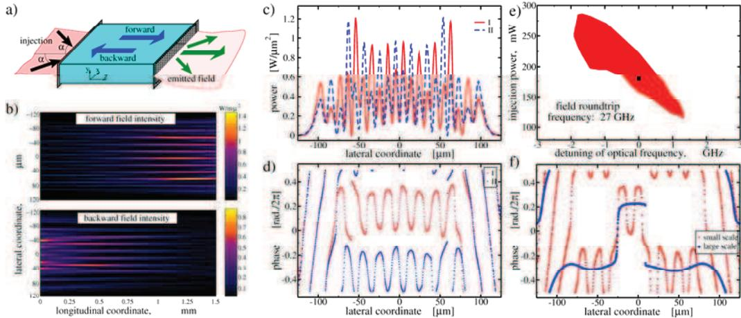
**Fig. 1** Evidences of spatial rocking in broad emission area semiconductor lasers: (a): the scheme; (b): the characteristic spatial field intensity distributions, representing one of two phase-locked states; (c): intensities and (d): phases of two different stable space patterns (near fields) due to the spatial rocking; (e): parameter domain of coexisting stable phase locked states. Black square indicates parameters used in panels (b-d); (f): phase soliton.
