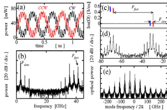
**Fig. 2** A dynamic regime induced by beating of different modes. (a): intensities of the emitted CCW and CW fields. (b): radiofrequency spectra of the CW field. (c): four main eigenvalues at several time instants. (d, e): optical spectra of the CW field. Parameters are as in Fig. 1(c), only  $\Delta_\beta \neq 0$ .
