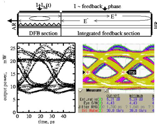
**Fig. 1** Top: scheme of a PFL, consisting of an anti-reflection coated DFB- and high-reflection coated IFB sections. Bottom: eye diagrams of simulated (left) and measured (right) response of the PFL to a PRBS current modulation (NRZ).
