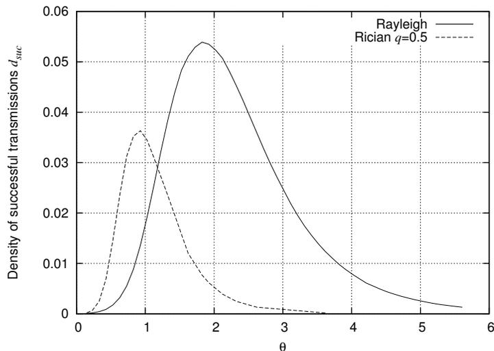
Fig. 16.4 Density of successful transmissions  $d_{suc}$  for Opportunistic Aloha in function of the deterministic threshold  $\theta$  in the Rayleigh and Rician (with  $q = 1/2$ ) fading cases; other parameters as on Figure 16.3.
