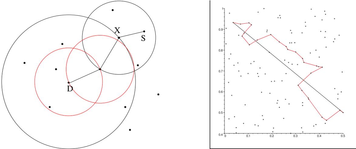
Fig. 20.1 Left: the next hop from point  $X$  on the route from  $S$  to  $D$ . Right: in red, the near-neighbor greedy route on a Poisson point process; in black, the straight line between the source and the destination, located in  $(.5,.5)$ .
