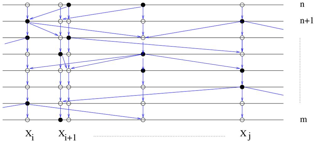
Fig. 21.1 The directed graph  $\mathbb{G}_{\text{SINR}}$  on  $\Phi \times \mathbb{Z}$ , where  $\Phi$  is a p.p. on the real line. The transmitters are depicted by black dots and the potential receivers by white ones.
