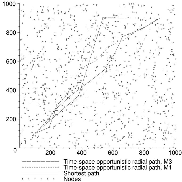
Fig. 21.2 Samples of packet paths with opportunistic radial routing (with and without fading) and of a MWR algorithm.
