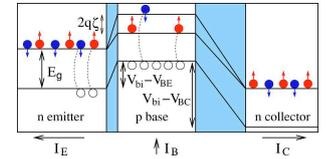
flows. If the relative orientation is antiparallel (lower figure) the current drops significantly. Right: Scheme of an n/p/n magnetic bipolar transistor with magnetic base B, nonmagnetic emitter E, and collector C. Conduction and valence bands are separated by the energy gap  $E_g$ . The conduction band has a spin splitting  $2q\zeta$  leading to an equilibrium spin polarization  $P_{B0} = \tanh(q\zeta/k_B T)$ . Carriers and depletion regions are represented as in the left figure.
