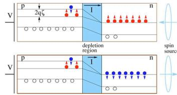
a magnetic bipolar diode. The p region (left) is magnetic, indicated by the spin splitting  $2q\zeta$  of the conduction band. The n region (right) is nonmagnetic, but spin polarized by a spin source: Filled circles, spin-polarized electrons; empty circles unpolarized holes. If the nonequilibrium spin in the n region is oriented parallel (upper figure) to the equilibrium spin in the p region, large forward current
