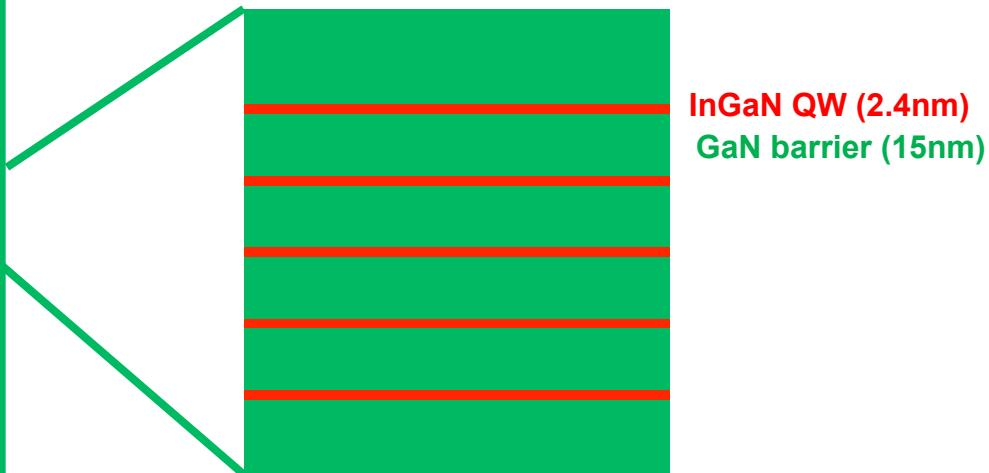
To analyze the model LED structure by TOF-SIMS inside the FIB/SEM, a typical Ga liquid metal ion source is unsuitable because it would inhibit the Ga identification from the GaN layers. Therefore we used a novel Xe plasma FIB.
