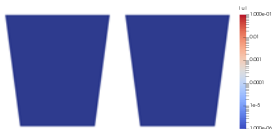
Fig. 3: Hydrostatic example with f(x, y) = \nabla(9.81y^\gamma) for \gamma = 1 (left) and \gamma = 6 (right), |\mathbf{u}| for a modified pressure-robust Bernardi–Raugel FEM [5]
