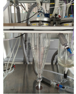
Fig. 4: An experimental fluidized bed crystallizer, built up by the Chair for Process Systems Engineering at Otto-von-Guericke Universität Magdeburg
