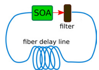
Fig. 3: Frequency swept FDML laser
