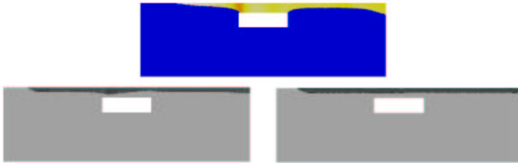
Fig. 1: Control of laser surface hardening to achieve a constant hardening depth: uncontrolled (top); linear PID subsurface control (bottom left); nonlinear PID subsurface control (bottom right).
